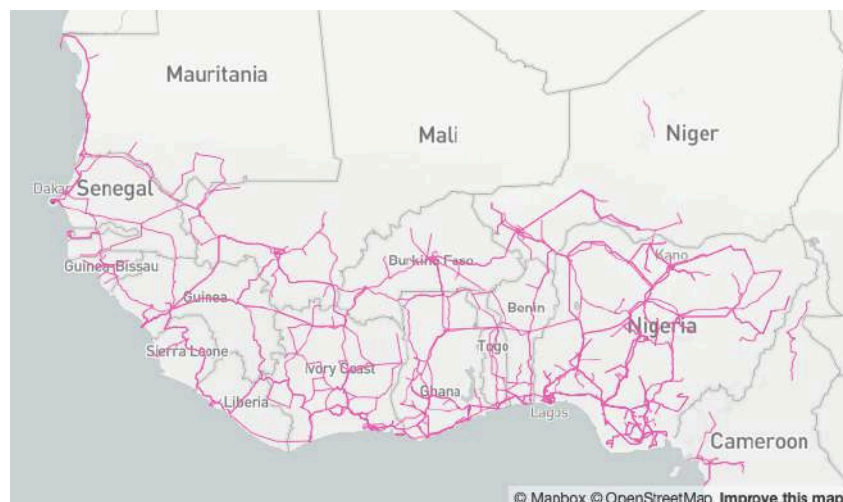
Figure 5.1.0: ECOWAS region existing and planning transmission grid network
