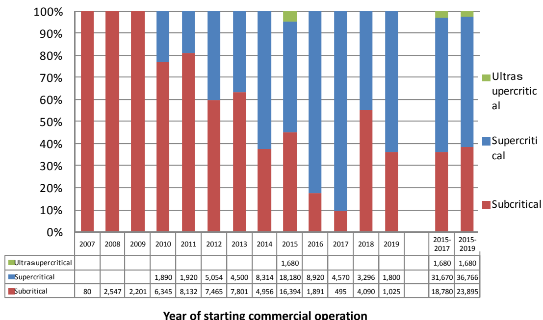
図 1 3 Types of boiler technology supplied by Chinese manufacturers and Alstom's Wuhan factory to overseas markets based on UDI World Electric Power Plants Database 2015 (March) (share)
